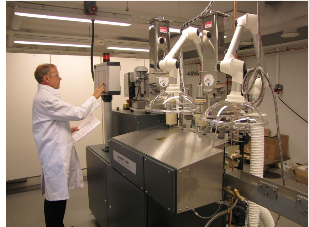
Twin screw extruder, throughput up to 150 kg/day
