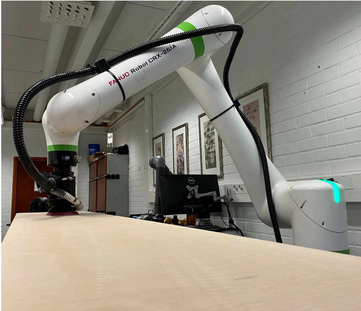
FANUC CRX-25iA cobot performing sanding operation at Centria University of Applied Sciences, Img. By: Ajay Sharma
