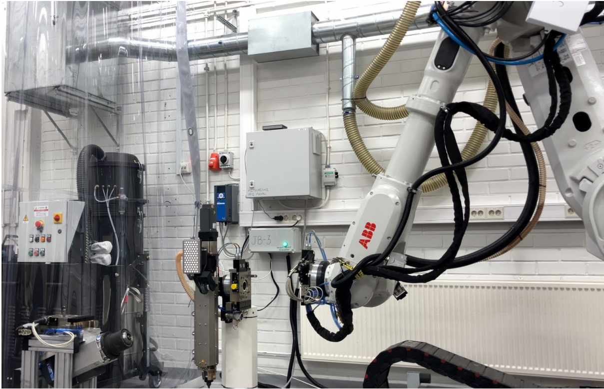
Robot while doing head changing process at Plast Lab, Img. By: Ajay Sharma
