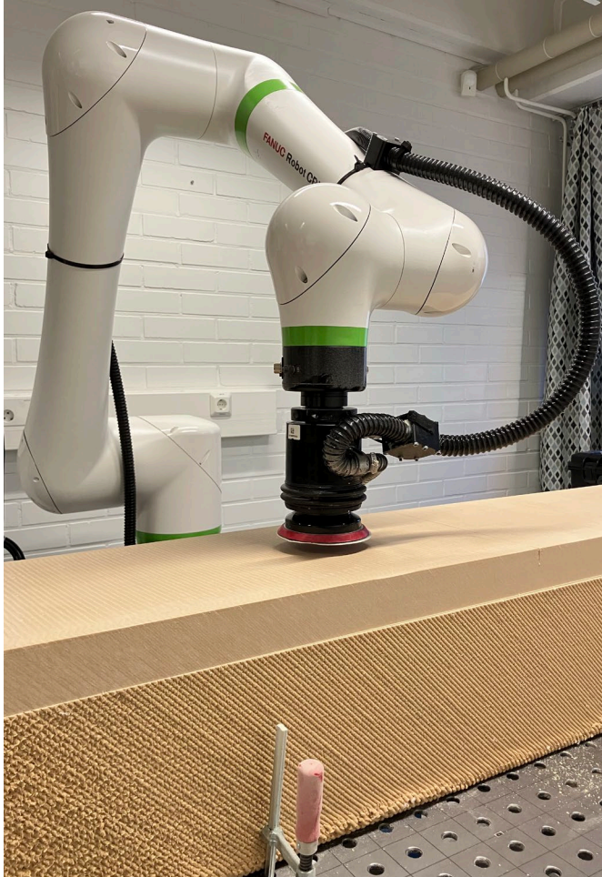
FANUC CRX-25iA cobot performing sanding operation at Centria University of Applied Sciences, Img. By: Ajay Sharma
