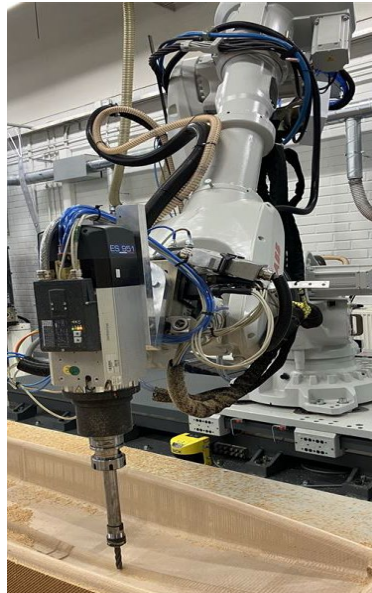
Robot milling in Plast Lab Img. By: Ajay Sharma
